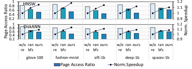
Fig. 14. Evaluation of static scheduling of NDSEARCH. Speedup is normalized to NDSEARCH without any reordering.
