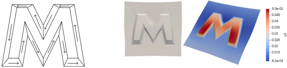
Fig. 14. Lifted M-origami : (Left) Lines indicate creases and arrows indicate the blueprinted director field \mathbf{m} in regions where \lambda < 1 , whereas \lambda = 1 within and outside the M. (Center and Right) Two views of final equilibrium configuration. Color on the right picture represents the value of y_3 and shows that the solid M and background are not completely flat.
