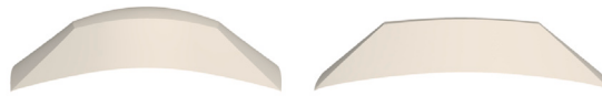
Fig. 10. Lifted square incompatible origami: The table shows a monotone decrease of discrete energy E_h[\mathbf{y}_h^\infty] and metric defect e_h^1[\mathbf{y}_h^\infty] in terms of h , which stabilizes to a positive value. Side views of the deformations for h = 1/128 (middle) and h = 1/64 (right). The buckling is more pronounced for smaller h .
