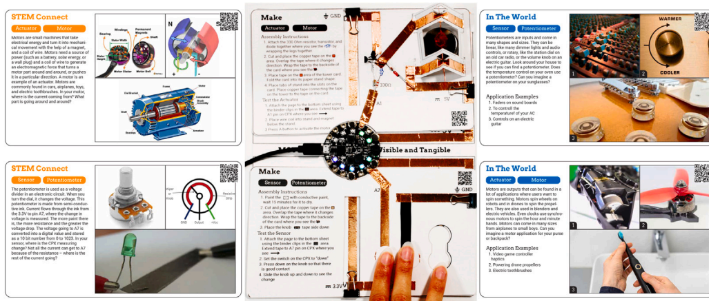
Fig. 1. MCVT card set example: (center) Base card layered with a visible and tangible potentiometer sensor input below and a motor actuator output above. (Left) “STEM Connect” and (right) “In the World” cards for each input and output are shown alongside.
