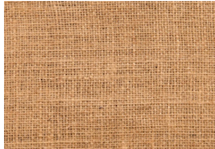
Figure 2. Plain weave woven jute textiles used as reinforcements in this study.
