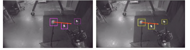
Fig. 11: Left : Left error vector (red) in left camera image calculated between features tracked in the magenta boxes, Right : Right error vector (red) shown in right camera image calculated between features tracked in the yellow boxes
