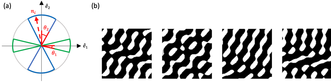
Fig. 2 Spinodoid topologies: (a) Schematic of the geometrical parameters: \theta_1, \theta_2 ; (b) Sample microstructures of 2D spinodoid metamaterials at \phi_0 = 0.35 in 128 \times 128 pixel resolution
