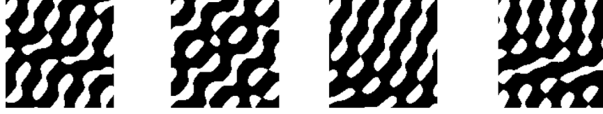
Fig. 2 Sample microstructures of 2D spinodoid metamaterials at \phi_0 = 0.35
