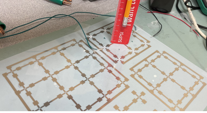
Fig. 4. Pencil drop experiment in the tactile sensor.
