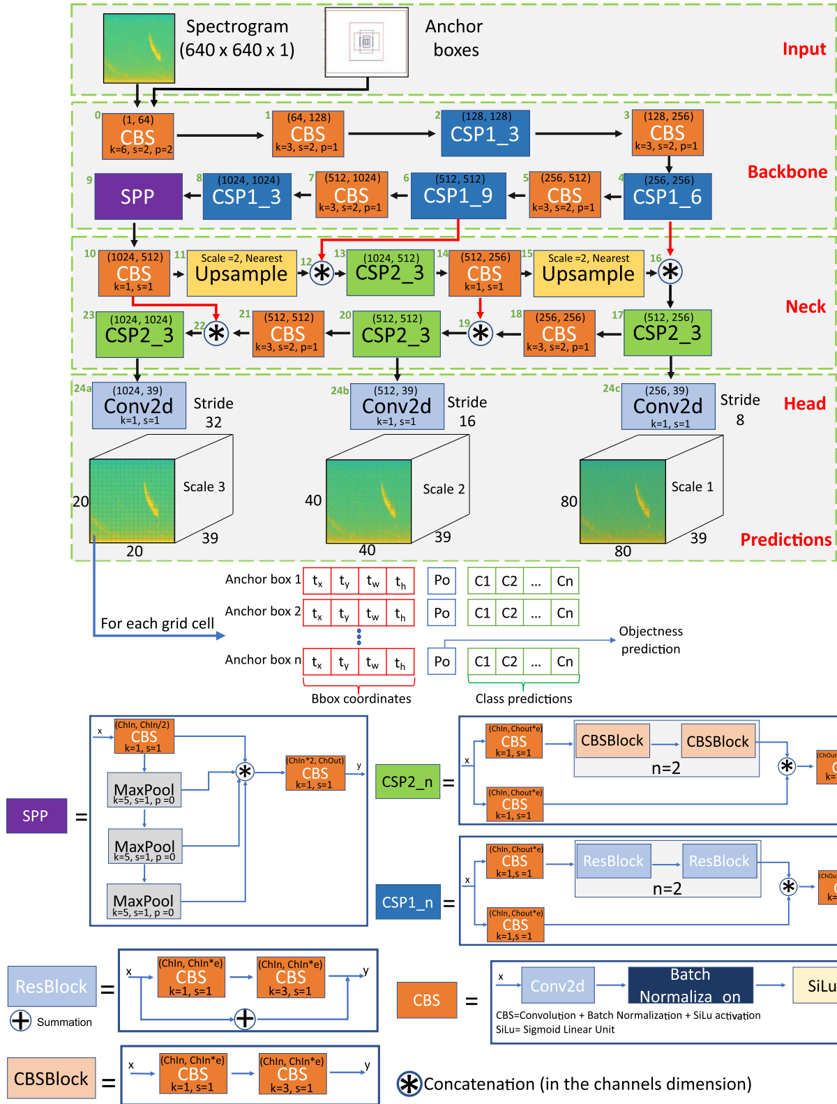
Fig. 3. YOLOV5 architecture. Numbers in parenthesis on top of each block represent the (input and output) number of channels. The kernel size ( k ), stride ( s ), and padding ( p ) are shown in the lower part of the CBS and Conv2d blocks. The green numbers in the upper left corner represent the layer number of their corresponding block. Asterisk blocks represent a concatenation in the channels dimension.
