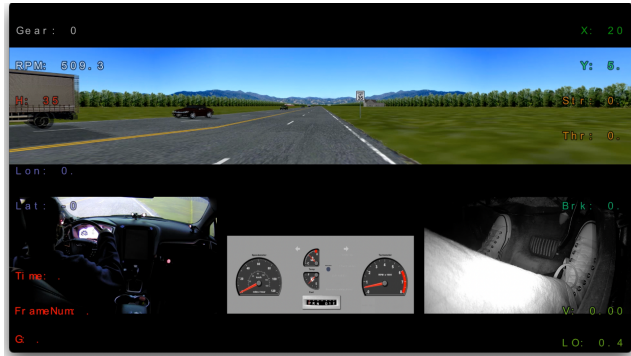
Figure 2: Camera view of hand and foot movements along with forward roadway and dashboard
