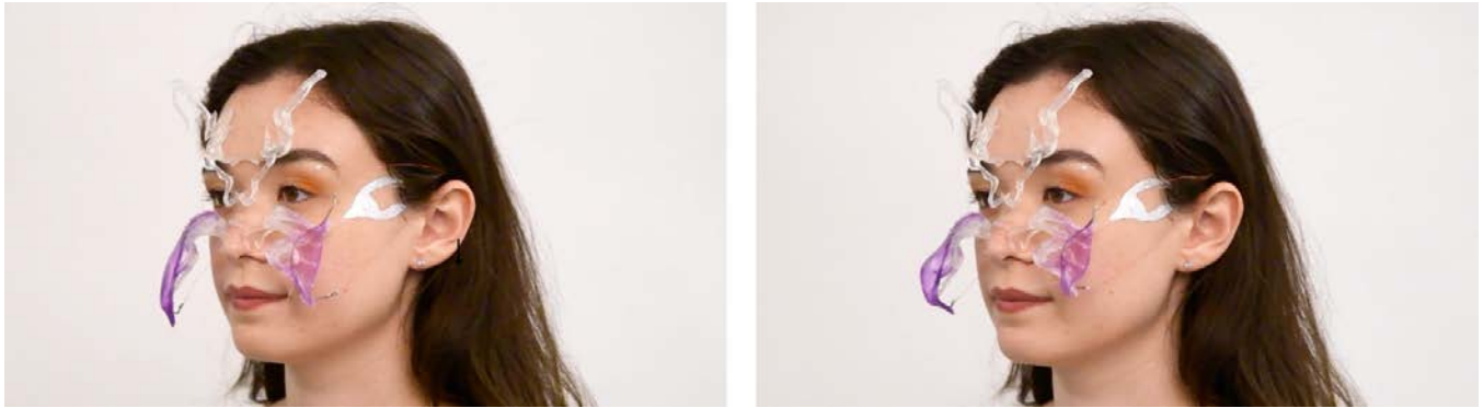
Figure 1: A model wearing the Social Prosthesis headpiece, nosepiece, and touch-sensing temporary tattoo. When the temporary tattoo is triggered through touch contact, the nose-piece starts curling in reaction.
