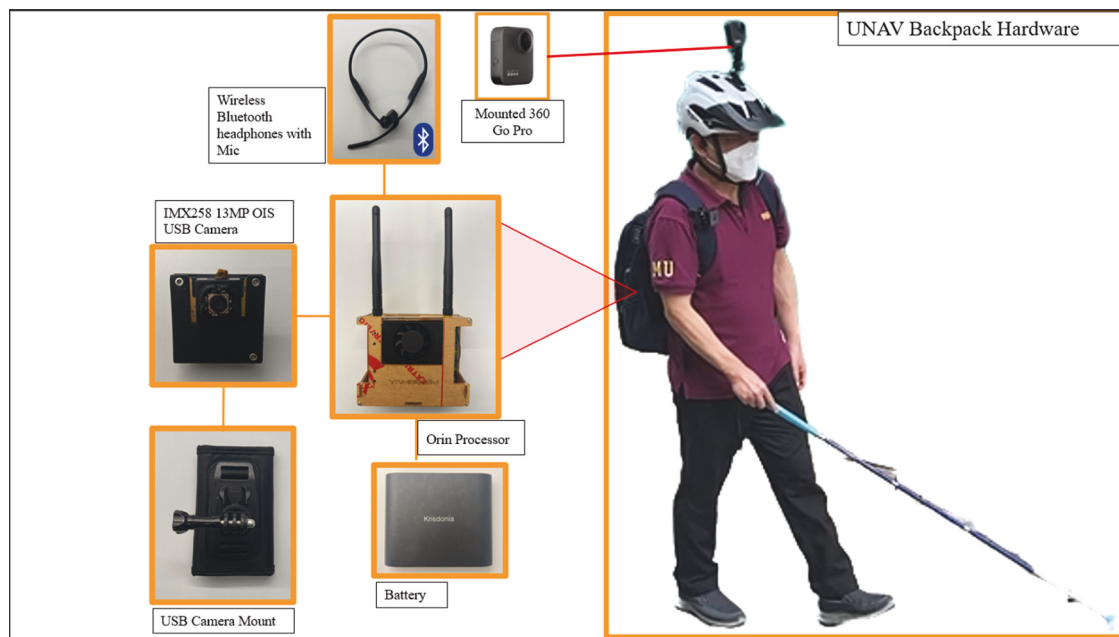
Figure 2. UNav system components housed in user backpack. Components supporting the UNav navigation system and data acquisition (left image), and how they are worn by the user (right image). Here we showcase the individual system components (orange boxes) and how they are connected to one another (orange lines). Local computational processing and networking is conducted by the Nvidia Orin board, which receives verbal input from the users' Bluetooth mic and images from a strap-mounted camera. This information is sent to a server for processing. Feedback is sent back by the server to the Nvidia Orin board and is then delivered to the user via Bluetooth to bone-conducted hearing.
