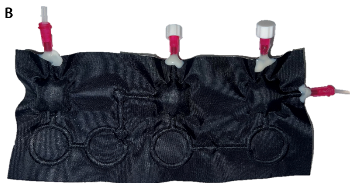
Figure S7. Modeled maximum volume of an arbitrarily sized inflated square plotted alongside the empirically determined volume of the textile cells. (A) Our cells match the expected volumetric function when filled with silicone elastomer at 1 bar of pressure. (B) The modified module is shown, filled with the elastomer. The measured volume is 17.58 mL for the entire module. When combining the volume of the cells and channels in the device, the average volume for the three cells becomes 5.86 mL, which puts the effective characteristic length of the cell at 31.3 mm as shown in (A).
