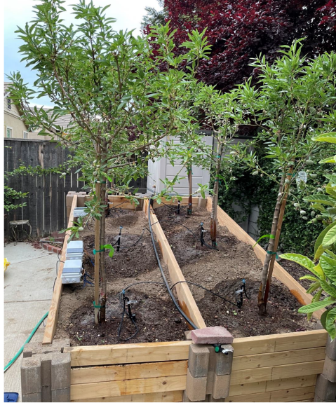
Fig. 8. Testbed and micro-sprinkler irrigation system.
