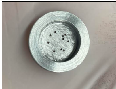
Figure 2. A manufactured prototype of the new NRM, with reduced dimensions and shaped for the Lyot wheel.
