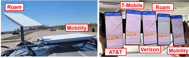
Figure 2: Two dishes are mounted on the rooftop and five smartphones are placed side by side in the vehicle.
