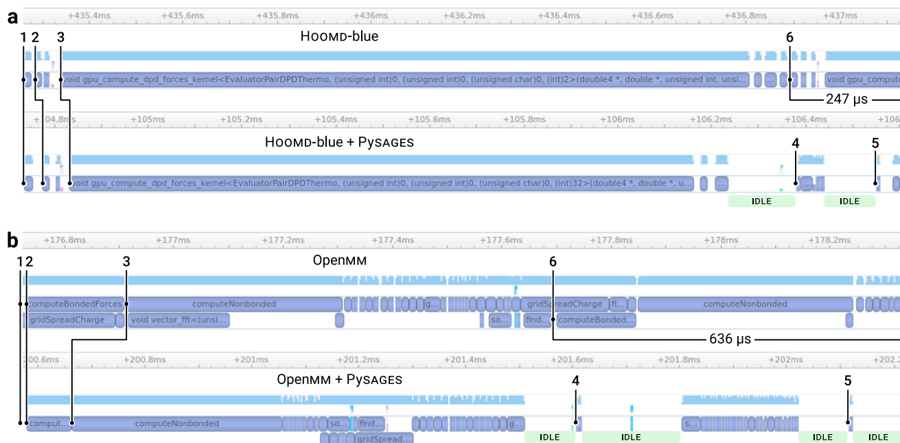
Fig. 9 Profiled timelines for a single-time step of unbiased and biased execution with HOOMD-blue and OpenMM. The profiles were recorded with Nvidia Nsight systems on an Nvidia V100 GPU. Light-blue represents the GPU activity while dark-blue represents individual CUDA compute kernels. The numbered lines indicate the same compute steps in all simulations: (1) start of integration step, (2) compute of bond forces, (3) pair-wise forces, (4) calculation of the CV, (5) addition of the harmonic biasing force to the backend, and (6) end of the integration step. (4) and (5) are PySAGES only and are executed on the GPU. We observe GPU idle time during the PySAGES Python coordination with GPU-JAX/CuPy (green bar), but note that there is no memory copies even within the GPU memory. a 1.8 ms of recorded HOOMD-blue execution. The top row shows a vanilla HOOMD-blue simulation step, while the bottom row shows a PySAGES/HOOMD-blue simulation with harmonic biasing of a center of mass CV. The additional time for CV biasing per time step is 247 \mu s. b 1.6 ms recorded execution time line of an OpenMM OPLS simulation of 40,981 particles as polymers with PME summation for long-range Coulomb forces. OpenMM works with asynchronous GPU kernel execution, which leads to less linearly-sorted timelines. Overall, the performance degradation is more pronounced with OpenMM compared to HOOMD-blue.
