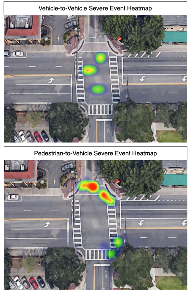
Fig. 7. The heatmaps for pedestrian-to-vehicle and vehicle-to-vehicle severe based on common conflict regions using both LiDAR and video streams using our system.
