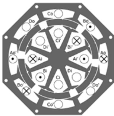
Fig. 9. Double stator SRM configuration.
