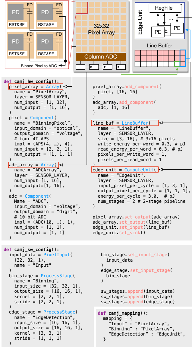
Fig. 5: An example of defining a simple CIS using the CAMJ programming interface in Python. The hardware architecture of the simulated CIS is illustrate at the top.
