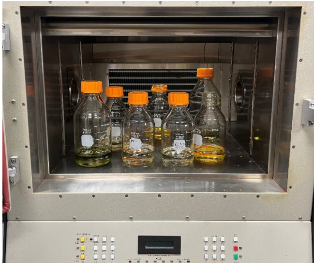
Figure 3: Sample bottles placed in a thermal chamber
