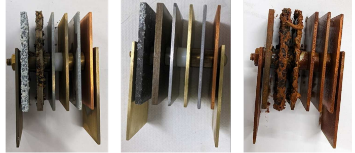
FIGURE 28: COUPON "BUNDLE" POST TEST FOR VENDOR A (LEFT), VENDOR B (CENTER) AND VENDOR C
