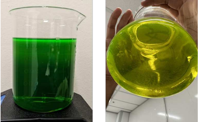
FIGURE 26: VENDOR B PG-25 COOLANT SOLUTION BEFORE TEST (LEFT) AND AFTER TEST (RIGHT)
