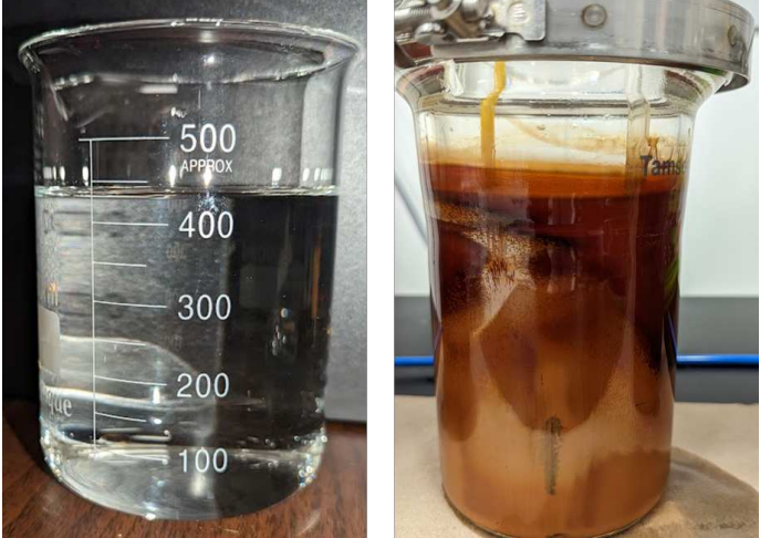
FIGURE 27: VENDOR C PG-25 COOLANT SOLUTION BEFORE TEST (LEFT) AND AFTER TEST (RIGHT)
