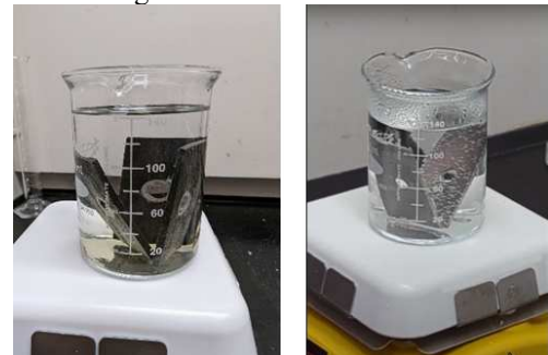
FIGURE 10: ALUMINUM COUPON IN \text{HNO}_3 (4:1) SOLUTION (LEFT), SOLDER COATED BRASS IN 1% GLACIAL ACETIC SOLUTION (RIGHT)
