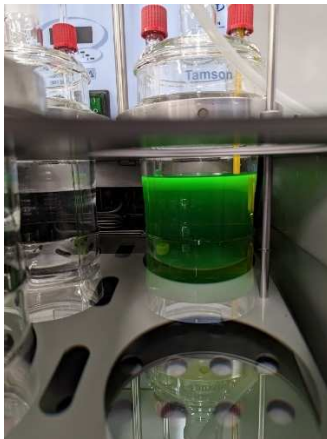
FIGURE 9: JAR PLACED IN THERMAL BATH OF ASTM D1384 APPARATUS
