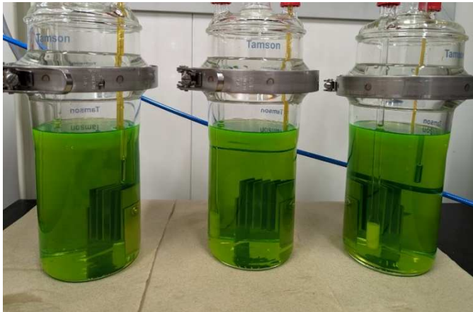
FIGURE 8: JARS WITH COOLANT SOLUTION WITH COUPON “BUNDLE” IMMERSSED
