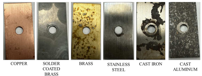
FIGURE 30: METAL SPECIMEN IMMERSSED IN PG-25 OF VENDOR A
