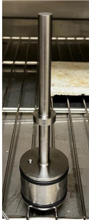
Figure 4. Piston Assembled with Set Screw and O-rings
