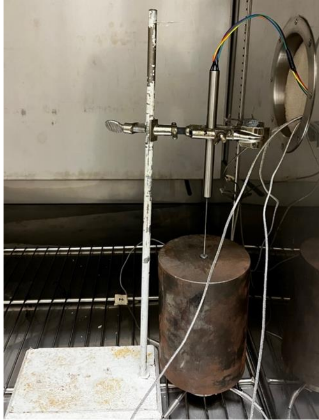
Figure 8. Placement of Piston-Cylinder Assembly underneath LVDT
