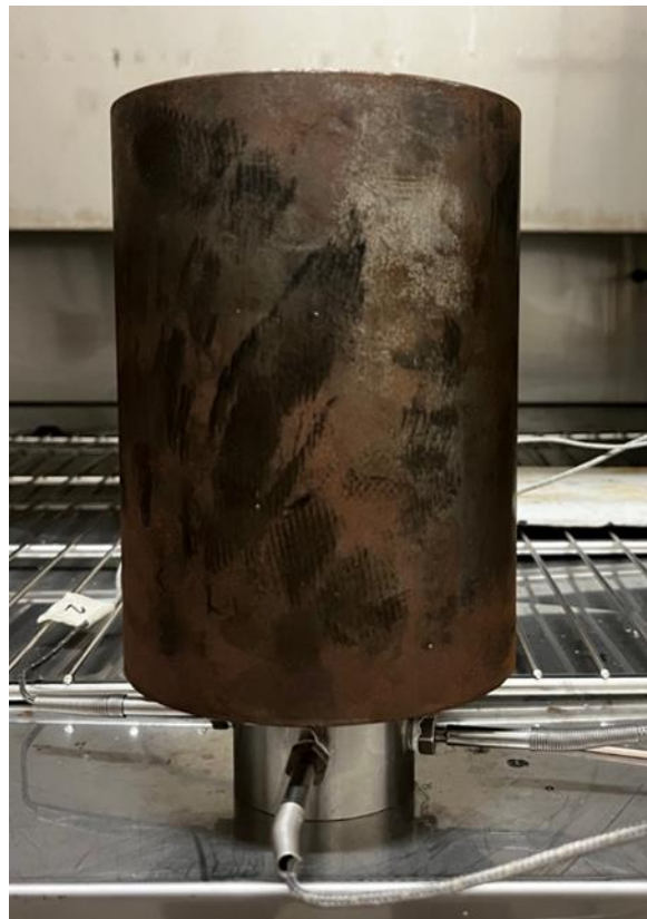
Figure 7. Test Setup After Installation of Piston and Weight
