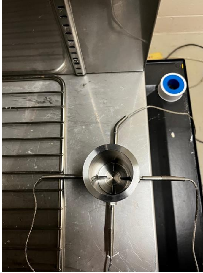
Figure 5. Thermocouples Installed into Cylinder
