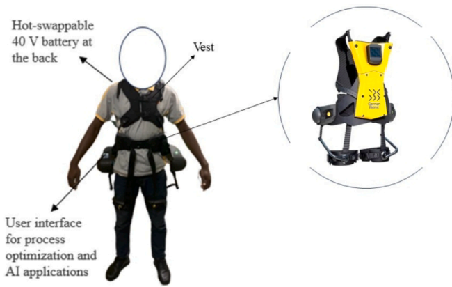
Fig. 3. Sample of the active back-support exoskeleton (CrayX).
