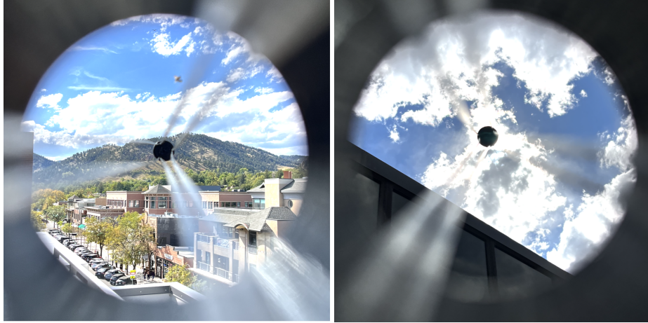
Figure 10. Initial test images taken through the CATEcor engineering unit reveal the geometry of the instrument front-end. Left: the Colorado front range above Boulder, CO; Right: the Sun with light clouds. These images were collected with a cell phone camera held at the aperture at the rear of the assembly. The truss is more strongly visible and the occulter appears slightly larger than in final images, because the cell phone effective aperture is much smaller than the full available aperture at the rear of the assembly.
