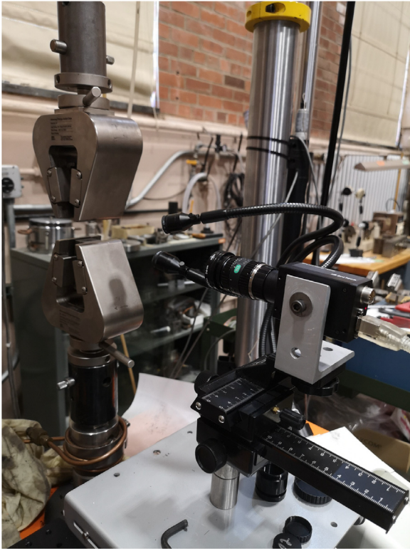
Fig. 2. Experimental setup for the tensile tests.
