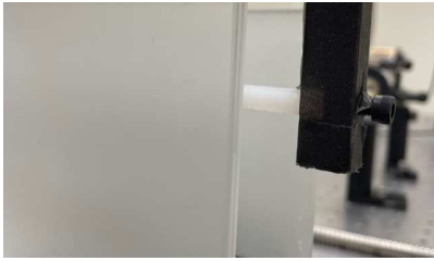
Fig. 3. Photograph of one of the scattering rods in the experimental setup. The rod is completely obscured from view by the stack of three ground glass slides, and the sample holder is kept out of the beam path.
