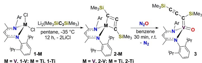
Scheme 2. Synthesis of complexes 2-M and trapping of the alkylidene-alkynyl 3 via oxidation with nitrous oxide (N 2 O) (Ar = 2,6- i -Pr 2 C 6 H 3 ).
