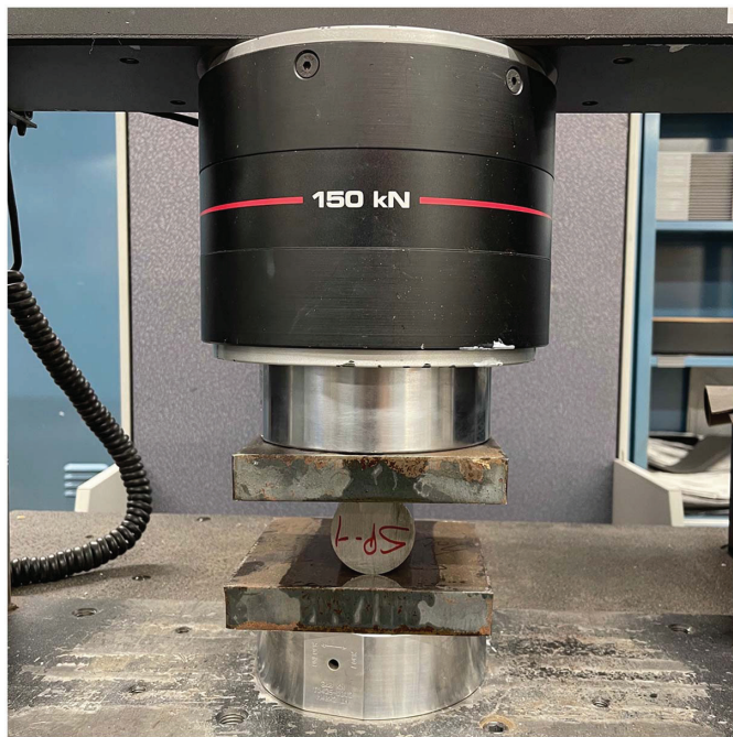
Fig. 13. Experimental setup for cylindrical contacting compression test.
