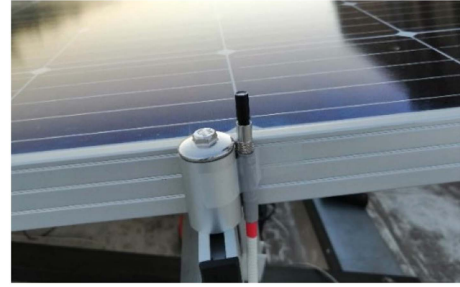
Fig. 5. Spectral measurement setup on the PV panels.
