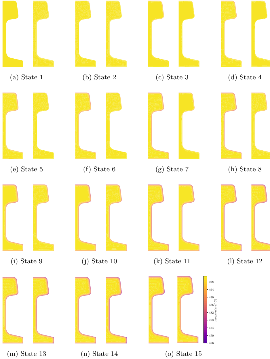
Fig. 6: Cooling of steel profiles (Section 5.1). High-dimensional states selected by sampling equidistant times (left) and by active operator inference (right) from the dictionary for n = 7 . For equidistant sampling, a majority of the states selected have cooler temperatures at the domain boundary with Robin condition. In contrast, active operator inference selects more states at the beginning of the cooling process, which leads to more accurate models in our experiments.
