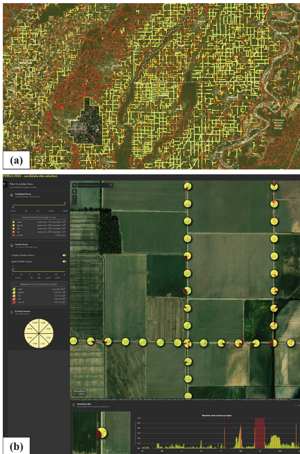
FIG. 4. Site selection tool. (a) Large-area view illustrating site-rich/poor regions as rated based on lidar mapping, with good sites colored green, through poorly rated red sites. (b) Small-area view illustrating pie chart sector-average horizon visibility scoring for sites spaced at 100-m intervals, and (bottom right) fine-azimuthal scale blockage scoring highlighting narrow blockage from, e.g., power poles and individual trees, and (bottom left) zoomed-in aerial view.
