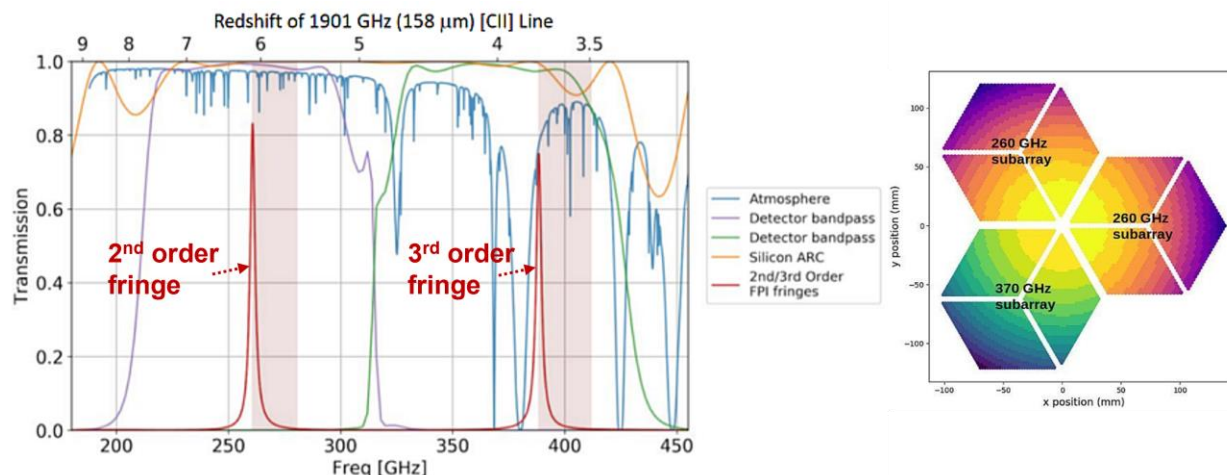
Figure 4. (left) Obtaining the spectrum over wide fields with EoR-Spec. Scanning is described in the text. Here we illustrate the case where the FPI is set at 260 GHz in 2 nd order for the on-axis beams, so it also resonates at 390 GHz in third order (red Lorentzian profiles). The pink shaded regions illustrate the spectral extent covered at this setting by other, more off-axis beams in the focal plane array. The two fringes are resolved from one another by detector bandpasses (purple and green near-rectangular traces) set by a low frequency pass filter in front of the arrays, and the high frequency pass filtering capabilities of the condensing cones. The blue trace in the background is the telluric transmission at 45^\circ elevation at the FYST site. The axis label at the top shows the redshift for [CII] line emission that corresponds to the frequency scanned as marked on the lower-level x-axis label. (right) The EoR-Spec focal plane. Two arrays are populated with detectors with bandpasses centered at 260 GHz, and the third is populated with detectors with bandpasses centered at 370 GHz. The higher areal coverage at 260 GHz is required by more challenging science demands of higher redshift line emission [18].
