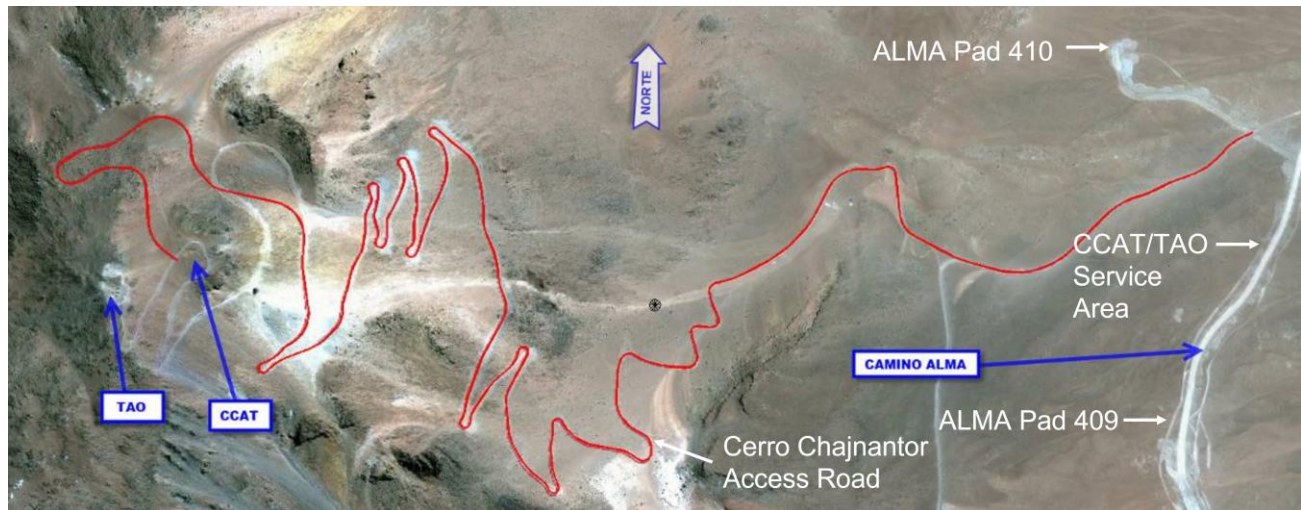
Figure 13. Site map. The red curved line is the upgraded road to the FYST and TAO sites from the ALMA road (right, white curves).
