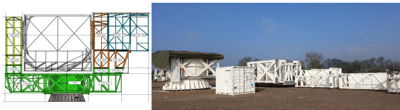
Figure 17. (left) Structure design of the FYST. The left and right yoke arms (light green and light red) and the yoke traverse (green) are manufactured and awaiting test fit assembly in Wessel (right).
