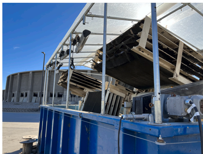
Fig. 2. A side view of the pilot scale RABR operating at the Central Valley Water Reclamation Facility (CVWRF). The algae biofilm is grown on a square substratum sheet and rotated into a 4,500 L tank containing anaerobic digester effluent. A plastic polycarbonate cover has been mounted to reduce heat loss in the winter months.
