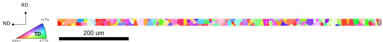
Figure 6. Uncleaned EBSD scan at 0.5 cycles in the 3x region taken across the entire sheet thickness. The left side is the bottom of the sheet. Noise on the right side represents the end of scannable material.
