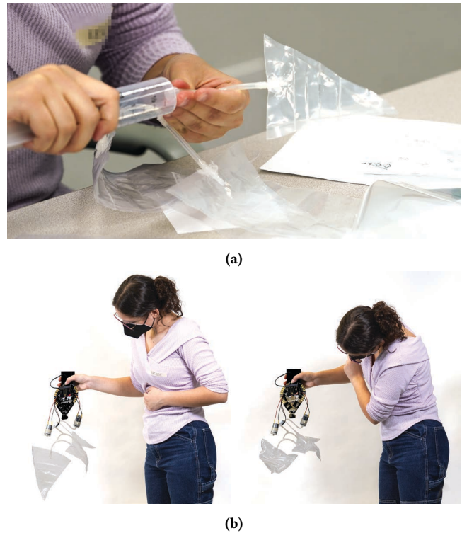
Figure 6: P4 working on her curve actuator. (a) She tests one module with the hand syringe. (b) She has hooked up several modules to the microcontroller pump. She directed the taking of these sequential images (deflated and inflated) and used them as part of her poster documentation.
