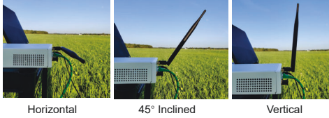
Figure 14: The three different antenna orientations.
