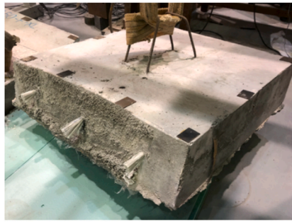
(a) PG14-450-F-XL: unloaded slab after failure
