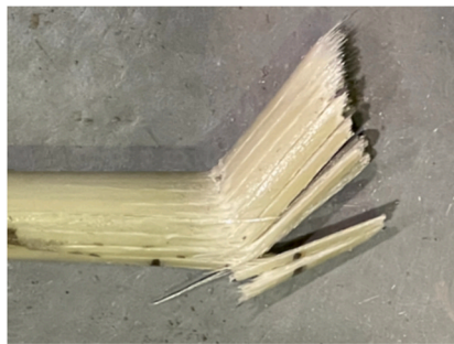
(e) shear failure in SG16 dowel bar
