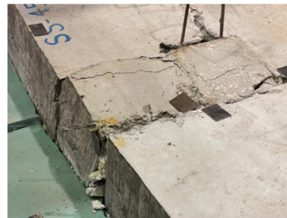
(f) SS12-450-F-XL: failure in loaded slab
