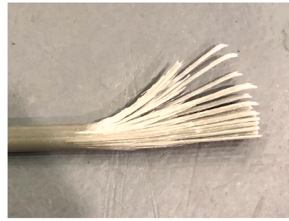
(b) PG-14 dowel failed in shear
