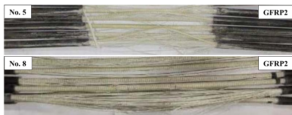
Fig. 8. Typical mode of tensile failure of the GFRP bars (No. 5 and No. 8).
