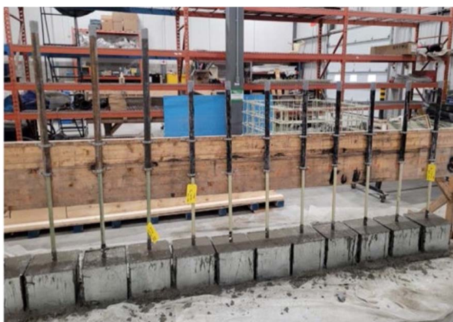
Fig. 6. Preparation of the GFRP bars for pullout testing.
