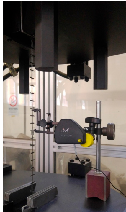
Figure 2. Direct tensile test on the BT.01 basalt fabric specimen.
