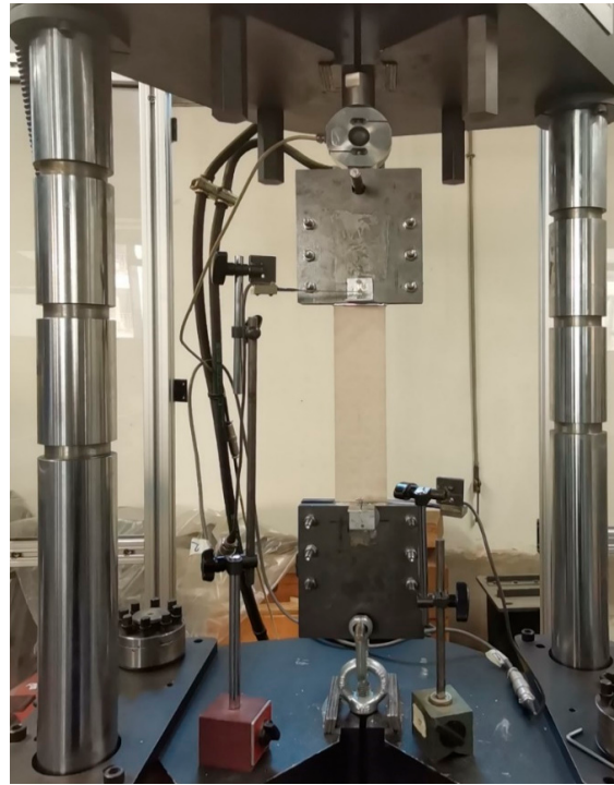
Figure 12. Direct tensile test on the FRLM coupon T-01.
