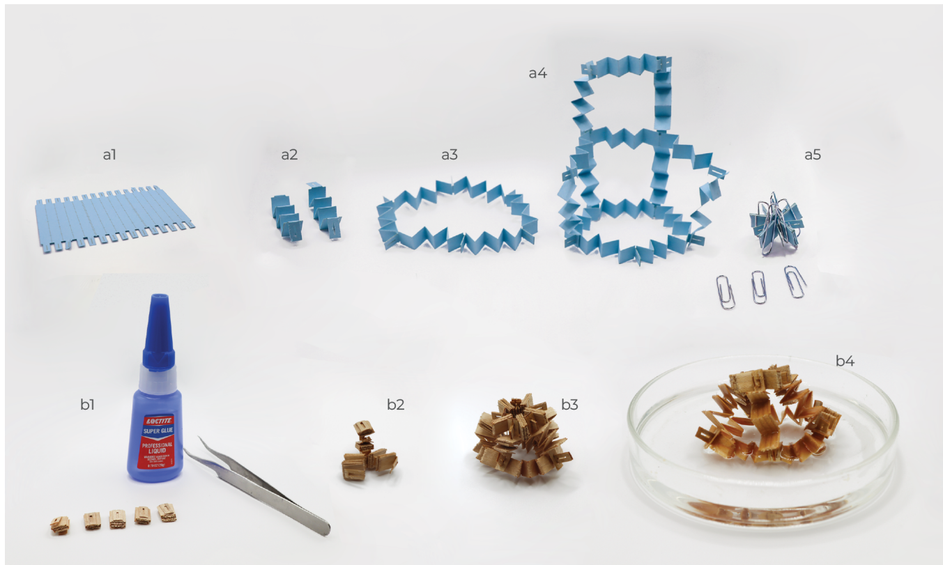
Figure 10: A. The design of ExCell lends itself to paper prototyping. Laser-cut models (a1) are folded (a2) and assembled into larger constructions (a3 and a4). To model the compressed state of ExCell structures, the paper models can be compressed with paperclips; B. The construction process of ExCell structures involves assembling discrete actuators together using glue (b1 - b3). Deployment can be tested in water (b4), and the structure can be re-compressed and dried for later use.
