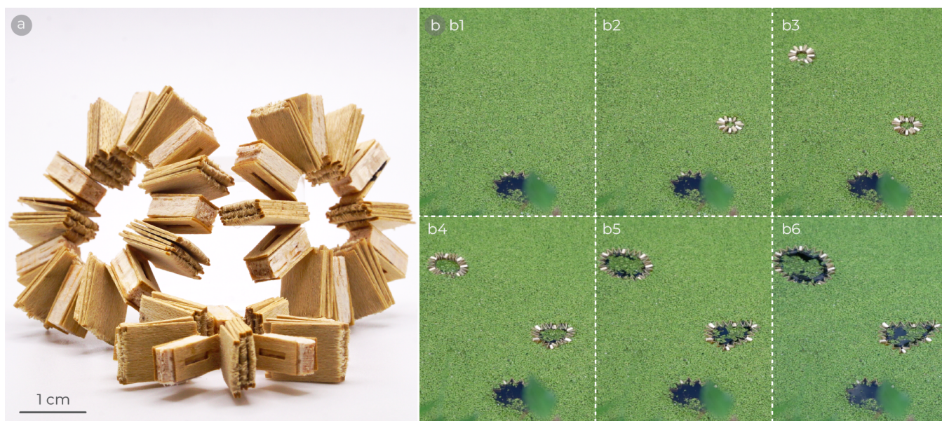
Figure 14: A. Three hand-deployable floating booms for creating oxygen and light-permeable voids in overgrown ponds; B. Timelapse stills of ExCell booms pushing duckweed away.
