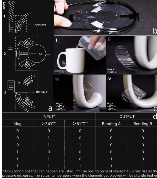
Figure 14: Responsive Mug Mat: (a) The digital design. (b) A closer view of the composites inside the mat. The white parts are heat-conducting silicone grease inside top layer chambers. (c) Different shape-changing outputs corresponding to different input conditions. (d) The truth table.
