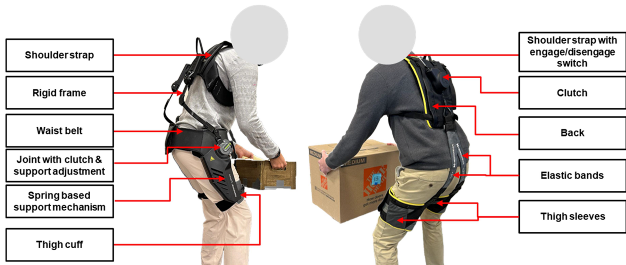
Figure 1. Paexo Back (left) and Herowear Apex (right) passive back-support exoskeletons with parts marked and labelled.
