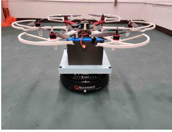
Fig. 4. Experimental multi-rotor on ground vehicle landing platform.
