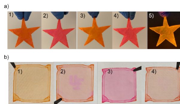
Figure 13. (a) Optical images of polystyrene films loaded with 0.1 wt % (w/w) 3a-Z: as-spun (1), after consecutive irradiations of 454 nm (2), 595 nm (3), 454 nm (4), and in a 365-nm UV light chamber (5). (b) Optical images of polystyrene films loaded with 1 wt % (w/w) 3a-Z: as-spun (1), after area-selective (2) or complete (3) 454 nm irradiation, and after 595 nm irradiation back to the Z-enriched PSS (4).
