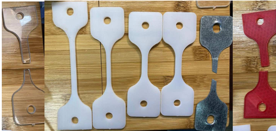
Figure 6. Various tensile samples used with the PUTM including polymer and metal samples.
