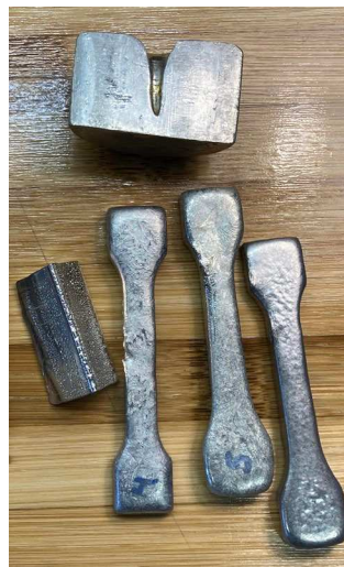
Figure 7. Various personal foundry casting samples showing shrinkage defect on the top.
