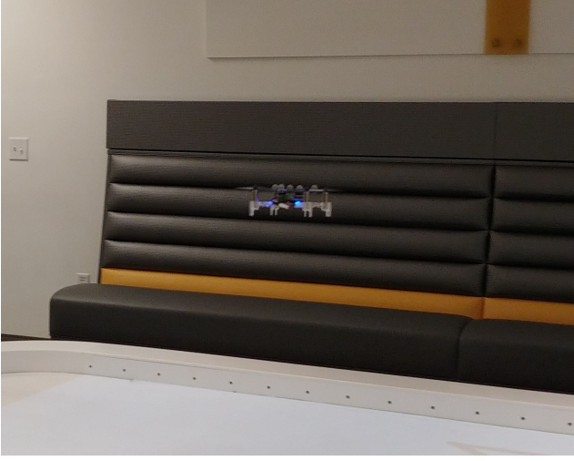
Fig. 4: A hardware demonstration of a Crazyflie nano quadcopter following a circular trajectory using our model predictive controller on ROS 2.
