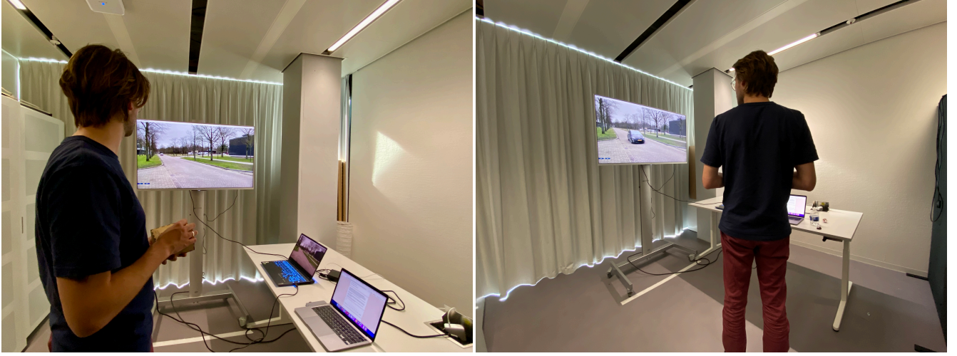
Figure 2: The setup of the experiment: the participant stood sideways in front of a 55" screen where the video stimuli were presented.
