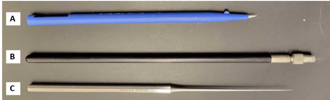
Figure 7. Tools used for removal of the vitelline membrane. (A) Stab knife for the creation of a slit towards the anterior end of the embryo; (B) Sharpened tungsten wire probe for removal of the anterior end of the embryo; (C) Roboz tool for extrusion of the embryo following removal of the anterior end of the embryo.
