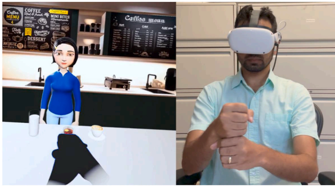
Fig. 7. A side-by-side view of the system. The left and right sides show the VR and real-world views, respectively. The user is signing COFFEE, and the avatar is waiting to provide feedback.
